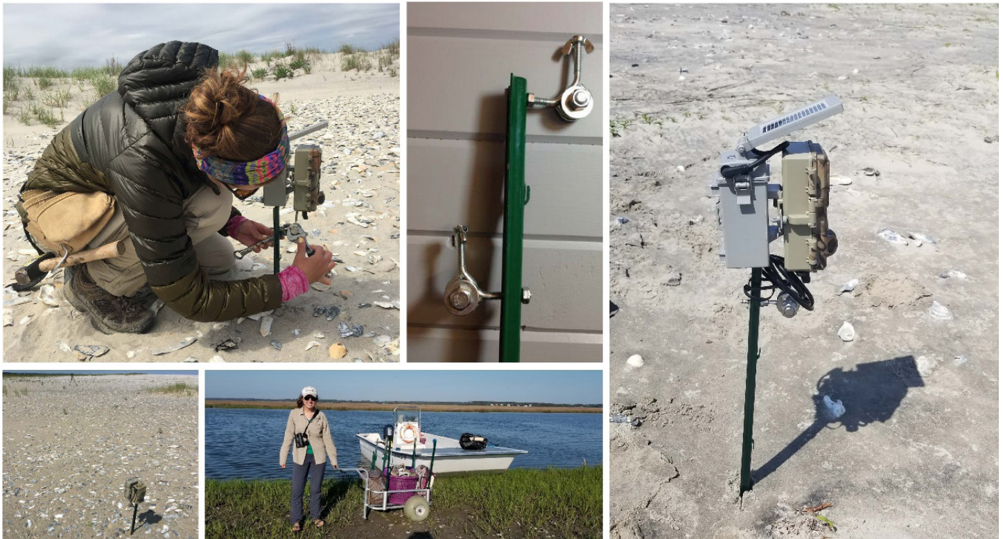
Figure 3. Top left, field installation of nest cameras. Top middle, DIY mounting bracket mounted on U-post (cambushcamo.com – note that our methodology used a single mounting bracket as opposed to double bracket shown). Right, deployed nest camera with solar panel. Lower left, deployed nest camera with nest. Lower middle, beach cart system for transporting equipment.
