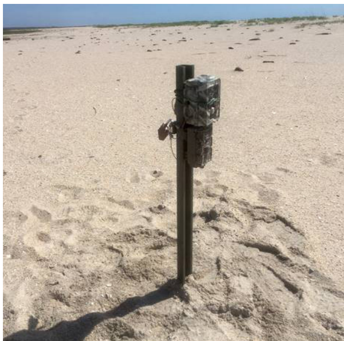
Figure 2. Typical two-camera nest monitoring system, deployed 0.6 meters above ground level, 3 meters from each nest. A Reconyx HC500 Hyperfire camera is on top and a Bushnell Trophy Cam HD (model 119973C) camera is below.
